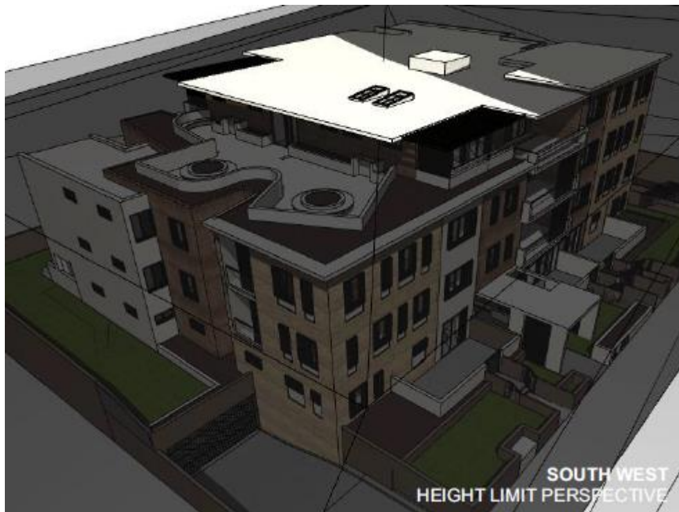
Figure 3.2 | Height Limit Breach in 3D provided by Ghazi Al Ali Architect.
